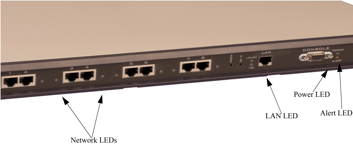
Figure 2-4 Front Panel LEDs
