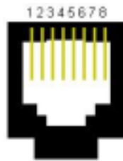
Figure 2-23 RJ-48 Port Pin Order
