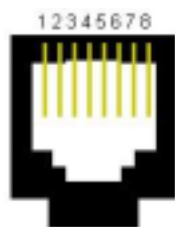
Figure 2-14 10/100 Ethernet Port Pin order
