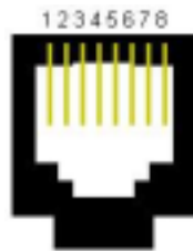
Figure 2-21 RJ-48 Port Pin Order
