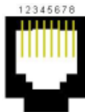
Figure 2-18 10/100 BASE-T Ethernet Port Pin Order
