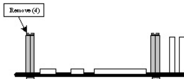
Figure 7-2 Remove four screws from exposed end
